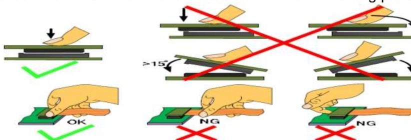
5. Precaution for soldering the LCM
