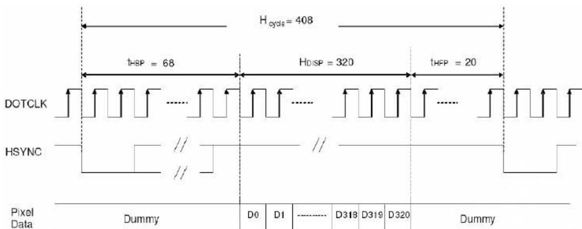
Horizontal data transmission timing (SYNC mode – Parallel RGB interface)
