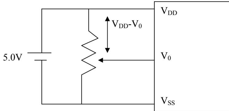
Where  $V_{DD}-V_0 = \text{LCD Driving voltage}$
