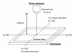
Fig.7-2 Optical measurement system setup
