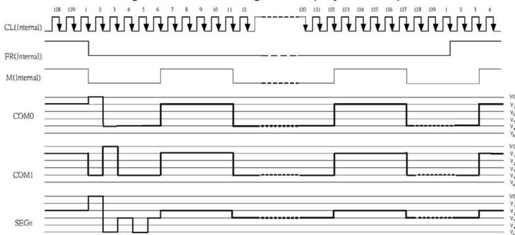
Figure 12 N-Line Inversion Driving Waveform (N=5,Duty Ratio=1/129)
