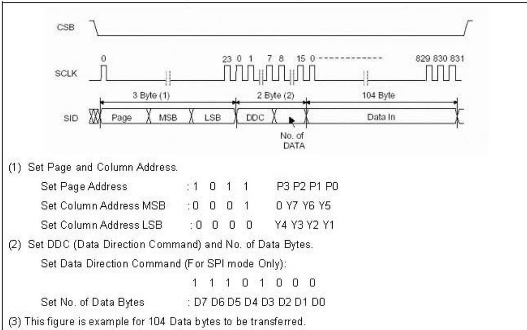
**Figure 2. 3-pin SPI Timing (RS is not used)**
