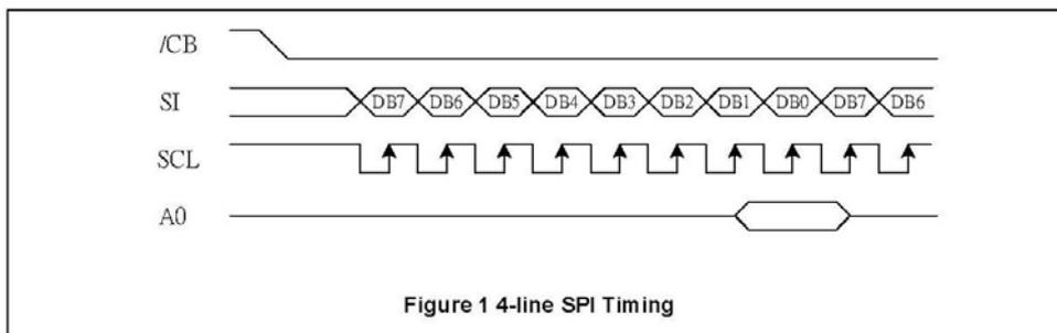
Figure 1 4-line SPI Timing
