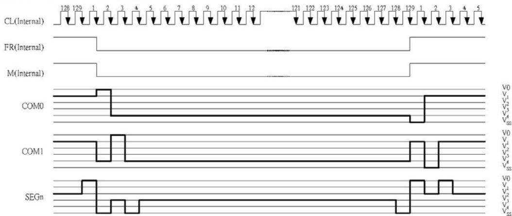
Figure 11 2-frame AC Driving Waveform (Duty Ratio: 1/129)
