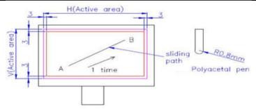
Operation force: 120g max (tip R0.8mm Polyacetal pen operation and R8mm silicon rubber, interval 2mm within Active area.
