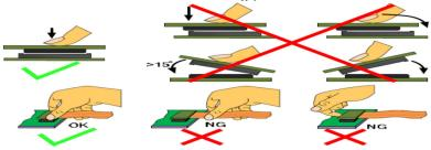
5. Precaution for soldering the LCM
