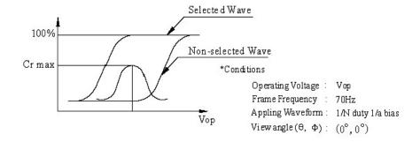
Contrast ratio (Cr) = <u>Brightness of selected dots</u> Brightness of non-selected dots
