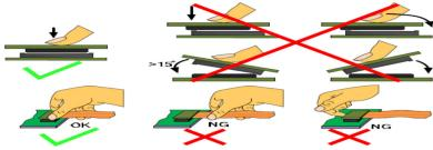
5. Precaution for soldering the LCM
