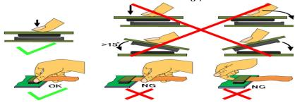
5. Precaution for soldering the LCM
