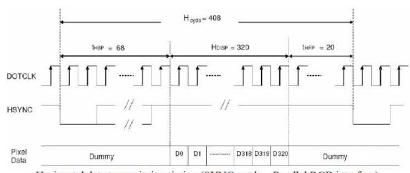
Horizontal data transmission timing (SYNC mode – Parallel RGB interface)
