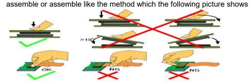
5. Precaution for soldering the LCM
