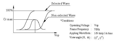
Contrast ratio (Cr) = <u>Brightness of selected dots</u> Brightness of non-selected dots
