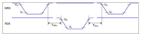
Write-to-Read and Read-to-Write Timing
