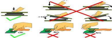
Precaution for soldering the LCM
