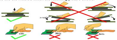
5. Precaution for soldering the LCM
