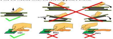
5. Precaution for soldering the LCM
