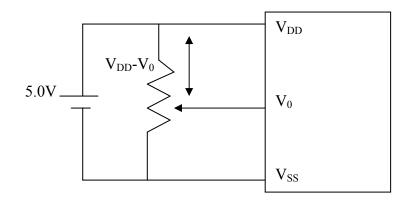
Where  $V_{DD}$ - $V_0$  = LCD Driving voltage
