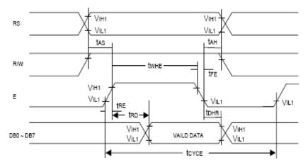
Figure 1. Bus Read Operation Sequence (Reading out data from NT7605 to MPU)
