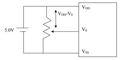
Where  $V_{DD}$ - $V_0$ =LCD Driving voltage
