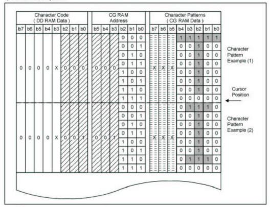
Note1: It means that the bit0~2 of the character code correspond to the bit3~5 of the CG RAM address.
