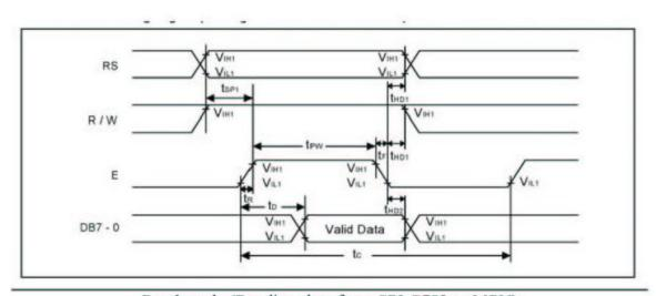
Read mode (Reading data from SPLC783 to MPU)
