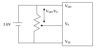
Where  $V_{DD}$ - $V_0$ =LCD Driving voltage
