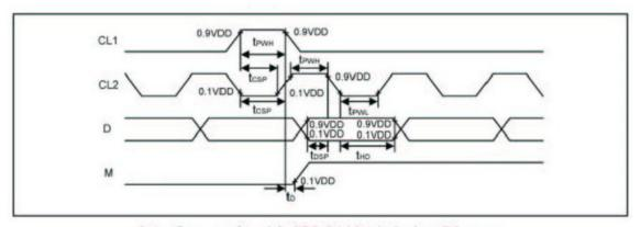
Interface mode with SPLC100A1 timing Diagram
