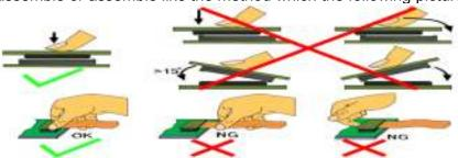
5. Precaution for soldering the LCM
