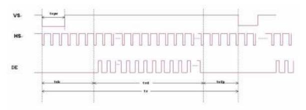
Horizontal Input Timing Diagram
