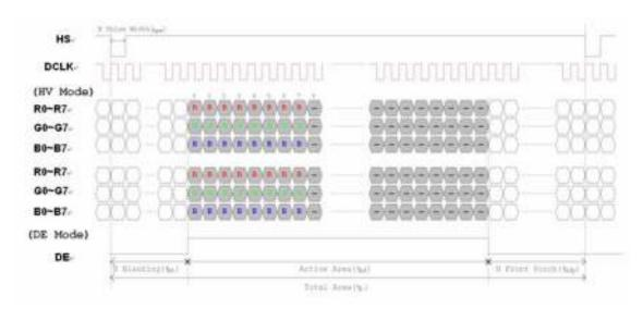
Horizontal Input Timing Diagram
