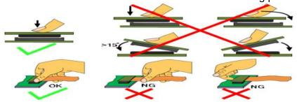
Precaution for soldering the LCM
