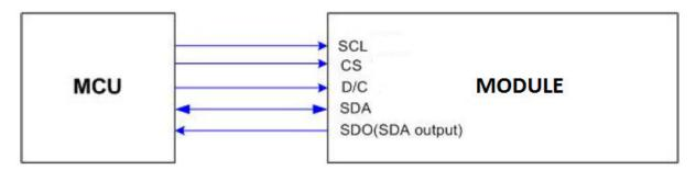
The 4-line/8-bit serial bus can be used by setting external pin IM [2:0] as 111.
