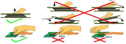
5. Precaution for soldering the LCM
