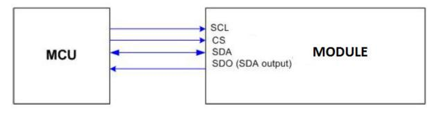
The 3-line/9-bit serial bus can be used by setting external pin IM [2:0] as 101.
