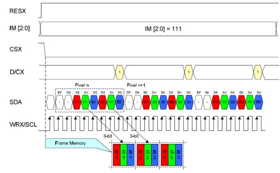
6.3.2.1 SPI Data for 3-bit/pixel (RGB 1-1-1 bits Input), 8 color
