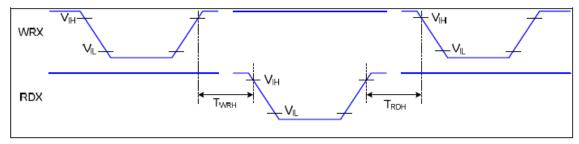
Figure Write-to-Read and Read-to-Write Timing
