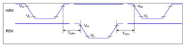
Figure Write-to-Read and Read-to-Write Timing
