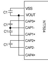
4x step-up voltage circuit  $~(C1=1.0\sim4.7~uF)$
