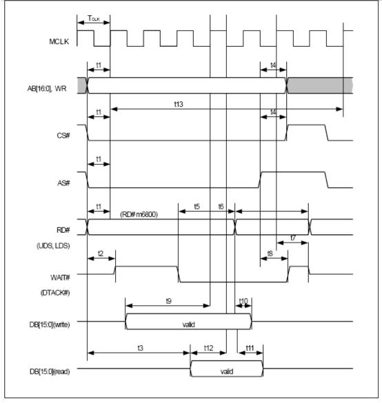
9.2 System Bus Read/Write characteristics (MC68K-series MPU)
